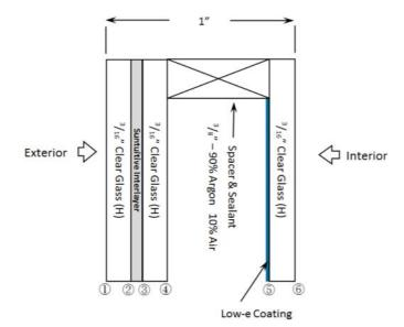
Suntuitive interlayer is laminated between two pieces of heat strengthened or tempered glass and placed into an insulated glass unit (IGU) with a low emissivity coating. A warm edge spacer is also recommended.
