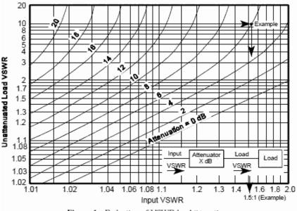
Figure 1. Reduction of VSWR by Attenuation
