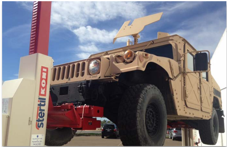
The new Stertil-Koni multi-purpose adapter is ideal for wheels free lifting, using only two mobile column lifts.
