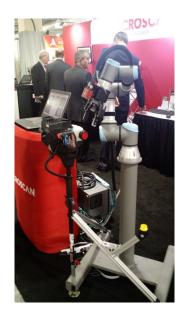
The UR3 robot demo was setup to read a Data Matrix 2D code and inspect the presence and position of several components on a small engine, such as
