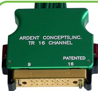
**Quick Latch** provides the same high standard of electrical performance as our Straight Mount configuration but adds the ability to mate and de-mate the TR quickly from the board by activating the red latches on either side. In a test & measurement environment, this makes the product much more user-friendly.
