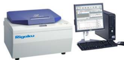
Rigaku NEX CG Cartesian geometry energy dispersive X- ray fluorescence spectrometer
