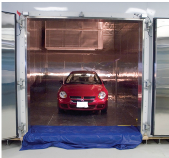
We feature combined temperature/humidity chambers with drive-in capability
