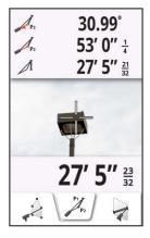
When the red-dot laser isn't visible outdoors, use the 4-power magnification camera with crosshairs to align your measurement point to the target.
