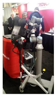
The UR3 robot demo is set up to read a Data Matrix 2D code and inspect the presence and position of several components on a small engine, such
