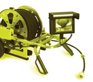
are less than 6 inches, and which have deteriorated or been relined multiple times. In such situations, it is difficult to maneuver a lateral launch system through the pipe, and inspection crews prefer using a jet-propelled drain camera (Fougerousse). These camera systems are essentially push cameras propelled by jetted water, and they have nozzles allowing them to steer through junctions and hover over debris. These cameras can successfully navigate
