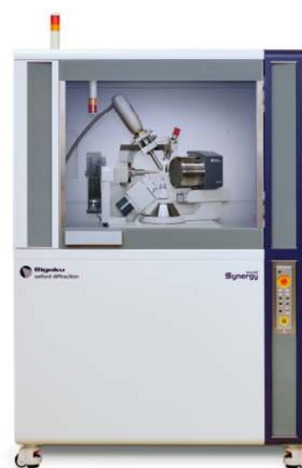
Rigaku XtaLAB Synergy single crystal X-ray diffractometer
