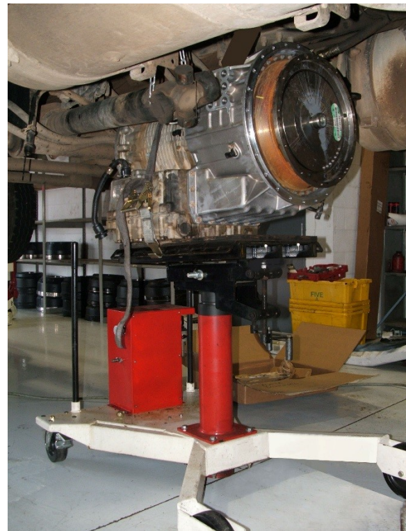
A Stertil Koni transmission jack is used to efficiently lift a transmission in a busy maintenance shop.
