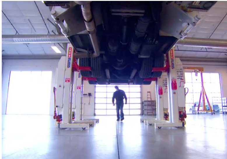
Wireless mobile column lifts are ideal for servicing heavy duty vehicles and eliminate the possibility of tripping hazards for the busy technician on the shop floor.
