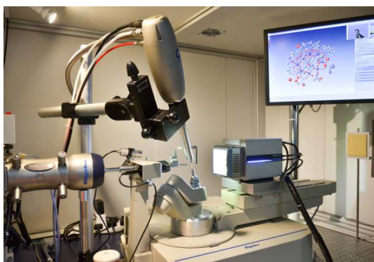
Rigaku XtaLAB FR-X DW X-ray diffractometer system in the School of Chemistry at the University of Manchester
