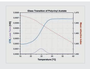
The mean refractive index curve (red dashed line) indicates the progress of volume expansion during heating.
