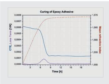
The mean refractive index curve (red dashed line) indicates the progress of the chemical conversion (curing) and volume shrinkage.
