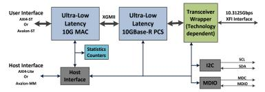
A complete reference design using a L2 (MAC level) packet generator/checker is also included to facilitate quick integration of the Ethernet IP in a user design. A GUI application interacts with the reference design's hardware elements through a UART interface (a PCIe option is also available). An application (with optional basic Linux PCIe driver/API) is also provided for memory mapped read/write access to the internal registers. See **Appendix A** for details.
