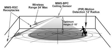
Note: For building spaces with lower levels and barriers, coverage size may decrease **Installation:** Easy mounting of adhesive pad and screws with the following placement guide:
