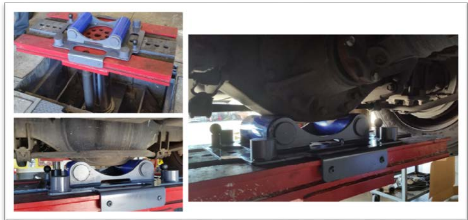
The differential adapter allows vehicles to be lifted by the “rear differential”; some people also refer to it as the “pumpkin” adapter
