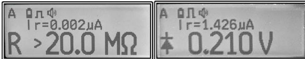
Diode mode is used for diode parameter extraction using DC bias. It is recommended for in-circuit characterization of p-n junctions. The screen displays the voltage drop in the open state when the forward bias is applied. If the reverse bias is applied, OL is displayed instead. Turn the jog-wheel counter-clockwise and hold for 1 beep to change the polarity of the probes.
