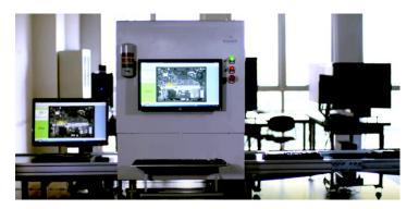
automated visual inspection station for in-line assembly verification. The INSPECT.assembly is fully-integrated with Radiant technology and configured to precise tolerances to meet production-level inspection needs of complex electronic assemblies. The INSPECT.assembly system detects the presence, position, and integrity of components including screws, cables, connectors, and other critical features before final device enclosure to automate assembly inspection.
