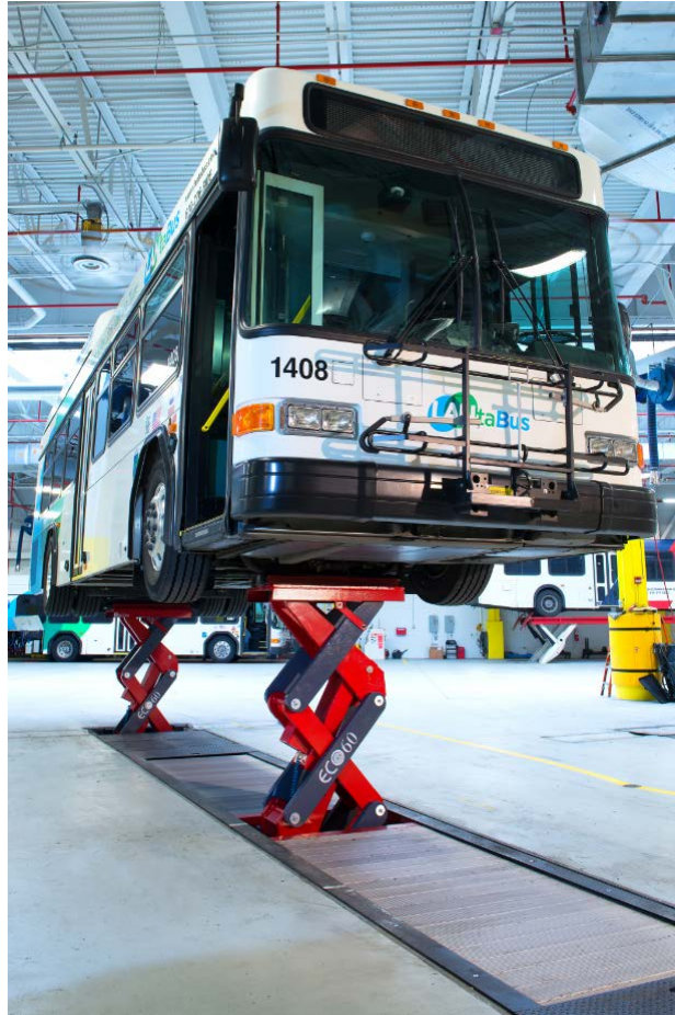
Stertil-Koni ECOLIFT at work, capacity 30,000 lbs. per piston
