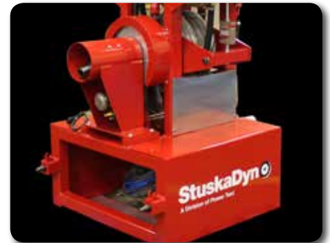
A more robust base and frame houses the XS-211-HD water brake for increased testing capacity
