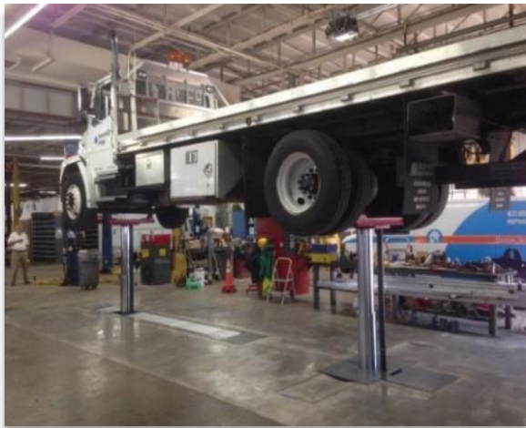
Stertil-Koni's DIAMONDLIFT requires a mere 4.5 gallons of biodegradable hydraulic fluid per piston
