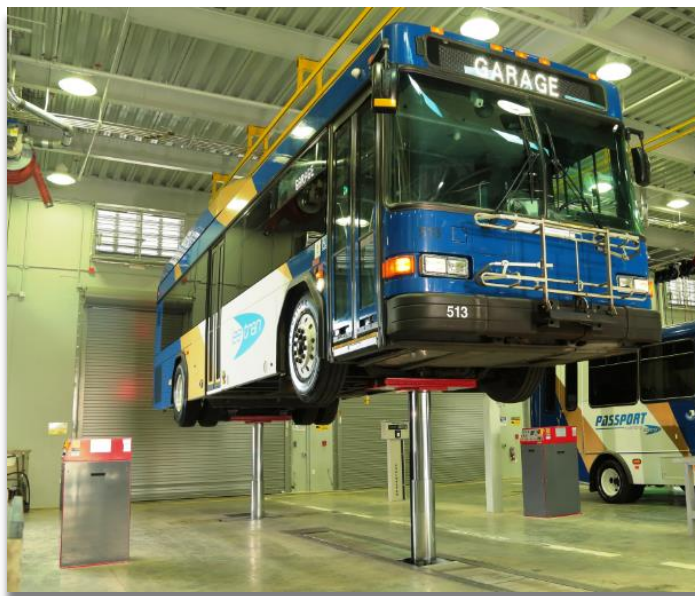
DIAMONDLIFT in two-piston configuration easily raises a transit bus
