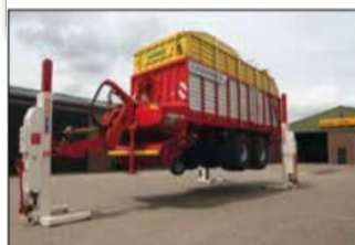
The agricultural multipurpose adapter is suitable for lifting tractors with two or three mobile columns
