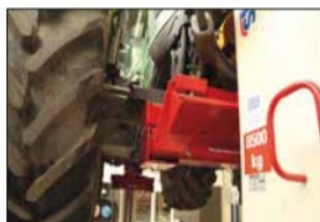
The agricultural multipurpose adapter is suitable for lifting tractors with two or three mobile columns
