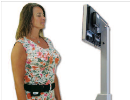
Vibrotactile cueing allows patients to get positional feedback with their eyes closed.
