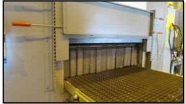
The work chamber of this conveyor oven is 3'6" wide x 25'0" long x 1'0" high. The continuous oven was designed with both top-down and bottom-up airflow to maximize heating rates and temperature uniformity of the part load configuration. The conveyor system utilizes a stainless steel flat wire belt and a variable frequency drive provides adjustable speed control.
