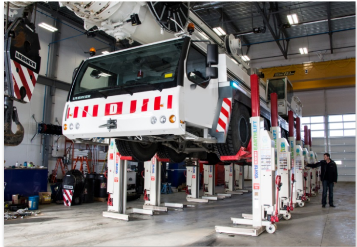
Wireless mobile column lifts are efficient, safe, and portable. They also minimize operator tripping hazards as there are no interconnecting communications cables
