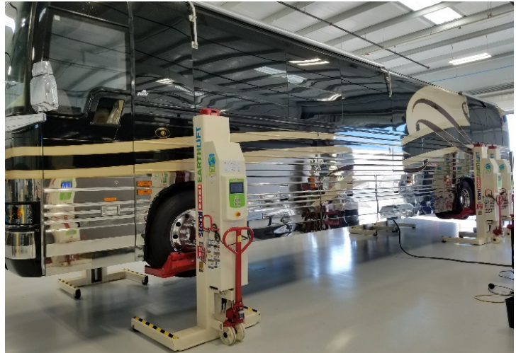
EARTHLIFT has an Active Energy Retrieval System (AERS) that delivers up to 50/5 more lifting cycles at maximum load
