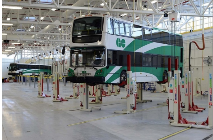
EARTHLIFT capacities range from 18,500 lbs. to 22,000 lbs. per column
