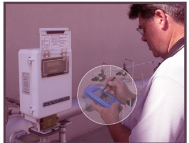
Operator using a PlantLog data collection terminal to record inspection readings.
