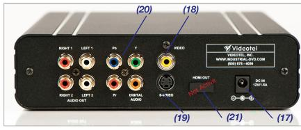
Component Video (20) - 3 RCA jacks (red/green/blue) in the middle of the player. All 3 of these connections can be used. They can also be used at the same time, in case you want to connect 3 TV's at once. The <a href="HDMI jack">HDMI jack</a> (21) on the back of the player is not available on this model. We don't have a unit currently available with HDMI output.
