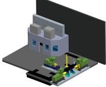
As part of the test system, RE offers complete data post-processing. RE Axle Test Systems also allow users to set accelerometer limits to detect early failure. These limits can be changed during scheduled tests or manual operation. A detected failure will either de-energize the system (coast stop) or command a controlled-ramp stop.
