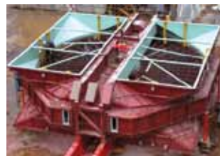
Howden 22m Dia. Rotary Heat Exchanger
