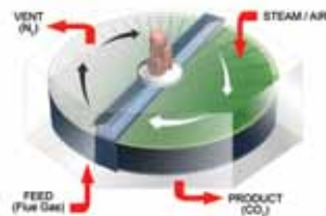
Structured Adsorbent Blocks are Assembled to form a Wheel
