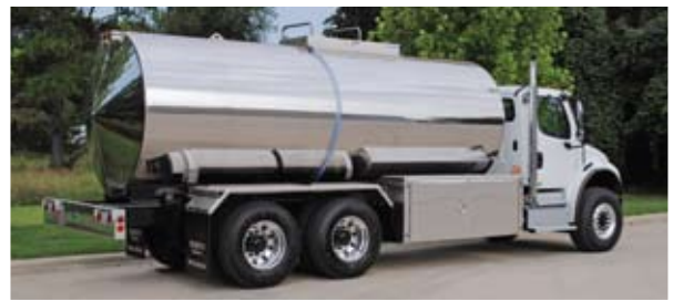
4000 Gallon Insulated & Heated DEF Truck
