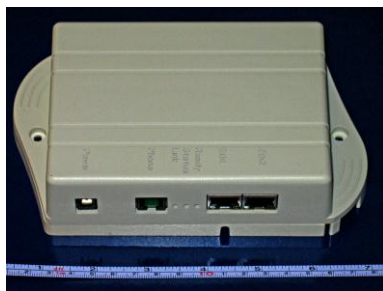
Access Point Connected to Telephone line
