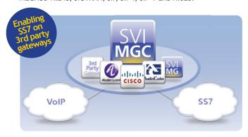
The globally deployed product enables clients to interface their VoIP networks to traditional SS7 PSTN based telephone networks allowing the rapid launch of VoIP services, NAS Modem Dial-Up and distributed networks with industry leading VoIP Media Gateways from Cisco, AudioCodes and Alcatel-Lucent.
