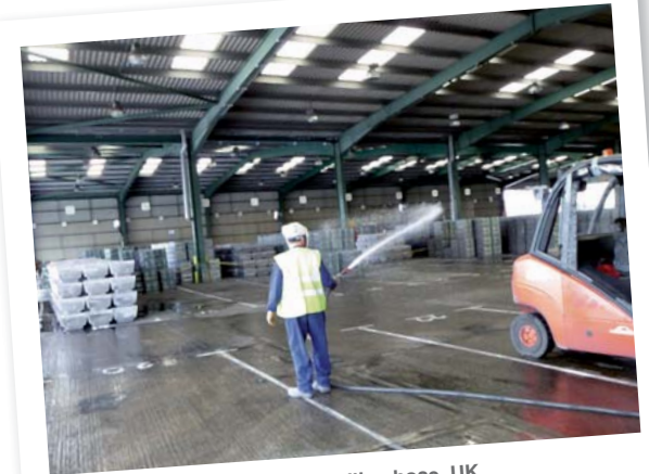
Damping down the work area with a hose, UK
