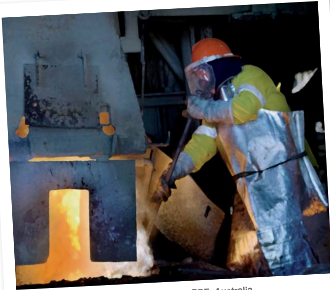
Tapping the furnace with the appropriate PPE, Australia
