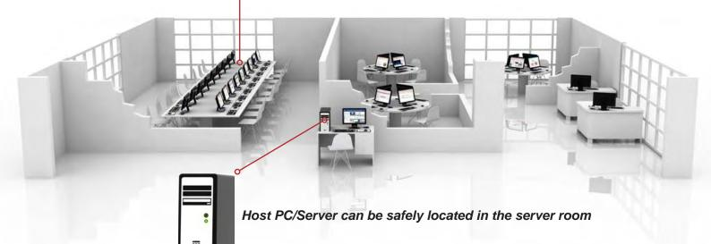
One standard PC with Core i7 processor and 16 Gig RAM can power 20 stations running independent 720p full screen videos.
