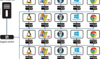
Zero client stations connect to the Host PC/Server over the LAN
