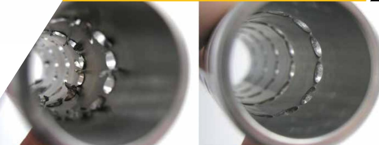
When deburring cross drilled holes using the Flex-Hone, it is helpful to first stroke and rotate the tool in a clockwise direction and then remove the tool from the bore, reverse the spindle and then stroke and rotate in a counterclockwise direction. This promotes a more symmetrical deburring pattern and prevents the burr from folding back into the cross-hole.
