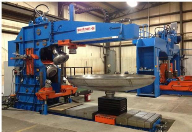
**Beaver Dam, WI (August, 2013)** — Apache Stainless Equipment Corporation, a manufacturer of stainless and carbon steel, and other high alloy ASME atmospheric vessels, announces the addition of new automated head making equipment.
