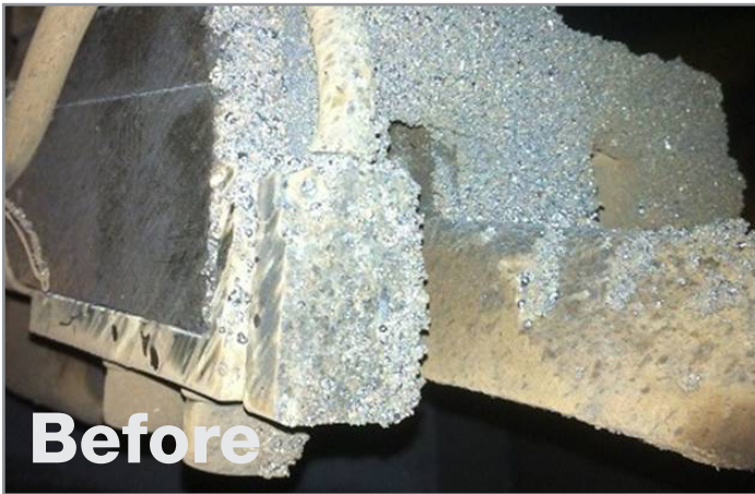
Weld spatter after one shift of production
