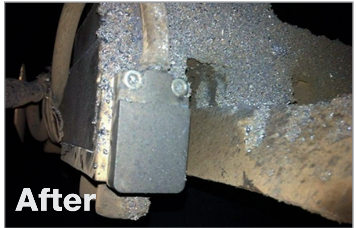
Sensor cleaned after one shift of production
