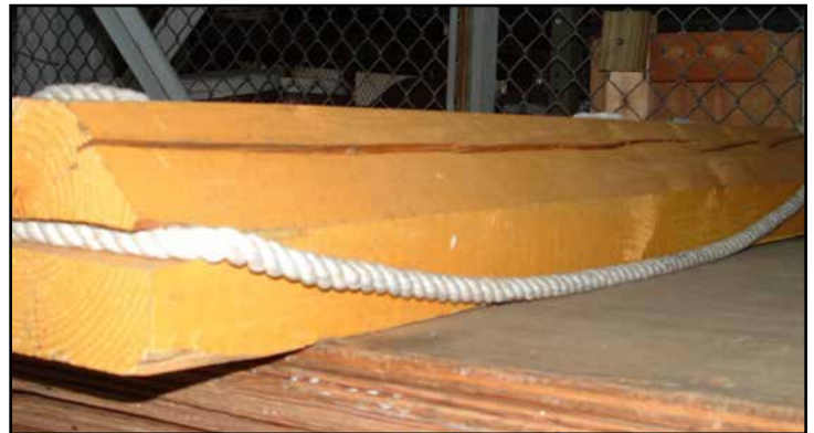
Wood Wheel Chocks tend to split and require regular maintenance, including painting.
