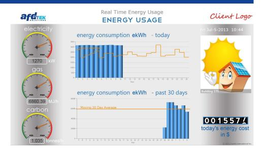
The AFDtek Energy Dashboard is designed to seamlessly integrate with any energy management system that supports the BACnet/IP protocol, OPC or the Johnson Controls Extended Metasys architecture. In fact, it can integrate with all of those architectures at the same time!
