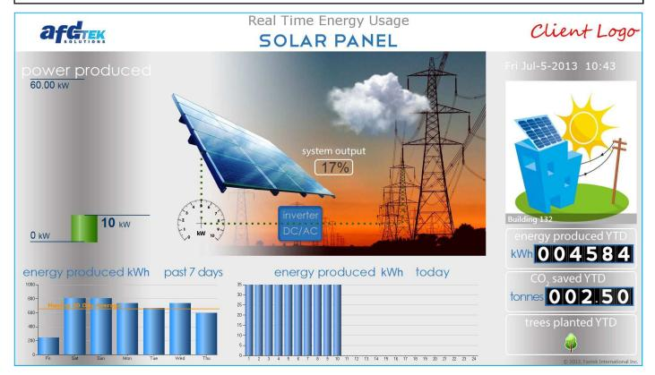
The Solar Panel page displays the maximum output, current output and "efficiency" of the current solar generated electricity production. These values are all mined from the energy management system. All other values are calculated by the dashboard from its stored data. The cloud indicates the current weather condition.
