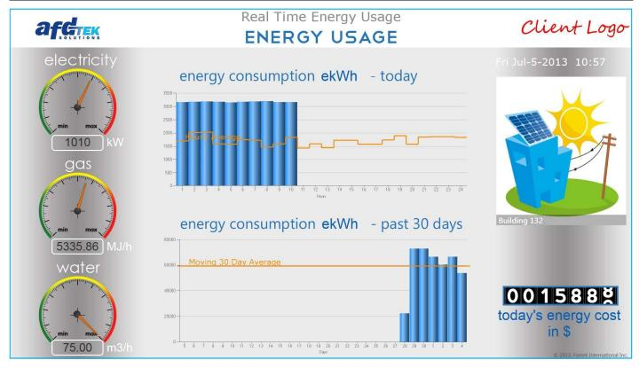
The Energy Usage page displays the current electricity, gas and water consumption. These values are all mined from the energy management system. The energy management system also provides the unit energy cost in dollars. All other values are calculated by the dashboard from its stored data.
