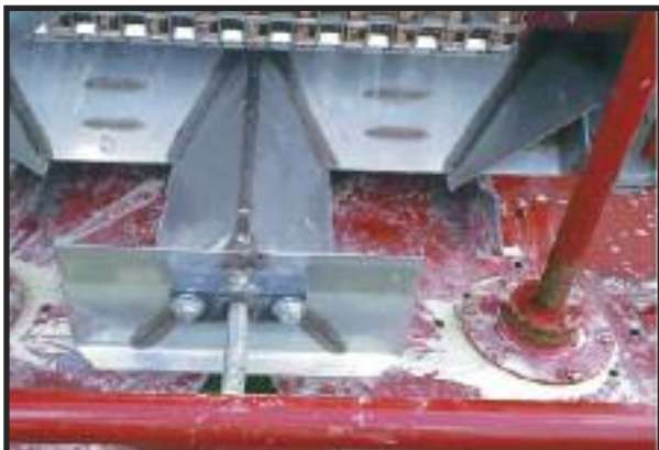
Making adjustments near the spreader gate to improve the distribution pattern
