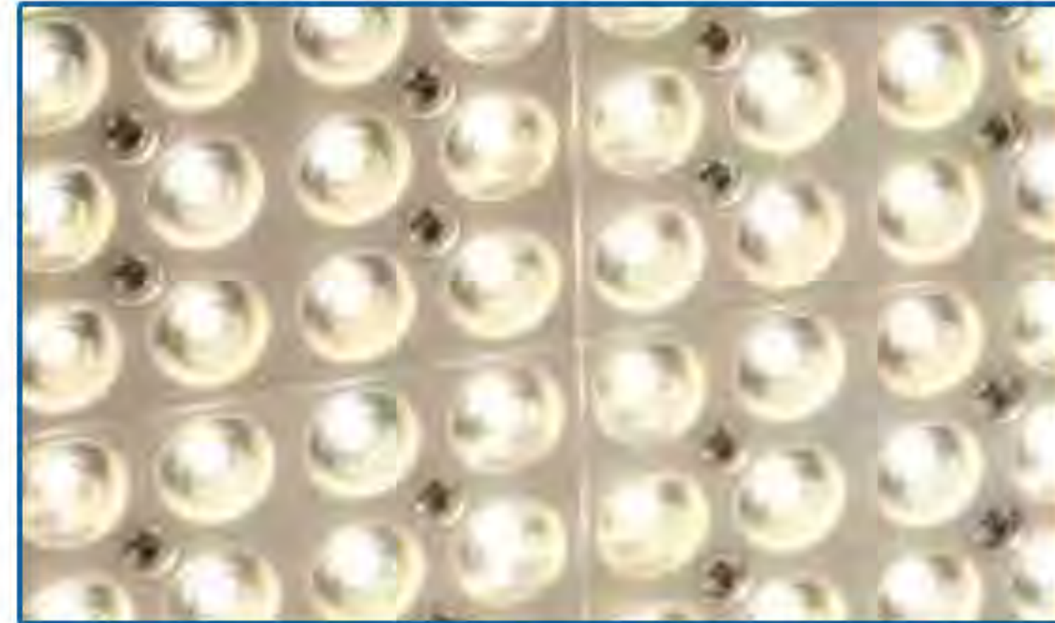
At one square inch per LED, the industry's largest spacing. More real estate per LED means less competition for the thermal pathway
