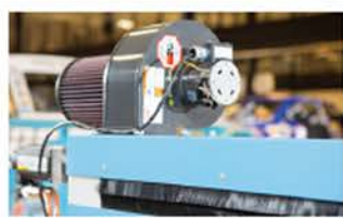
Motion components are protected with metal covers, seals and blower fans
