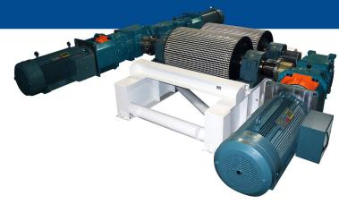
The image shown above is a triple 500HP Alignment-Free VFD Belt Drive that was shipped to a coal mine in West Virginia utilizing the ZHRH3-CRN/CLN-28, UniMiner Drives with high speed shaft fan and motor lantern for T10 coupling.
