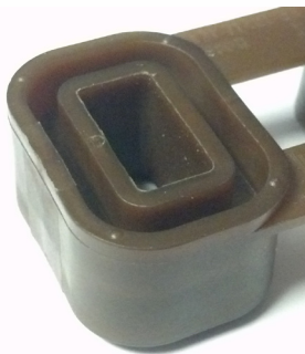
Missing gasket photo
