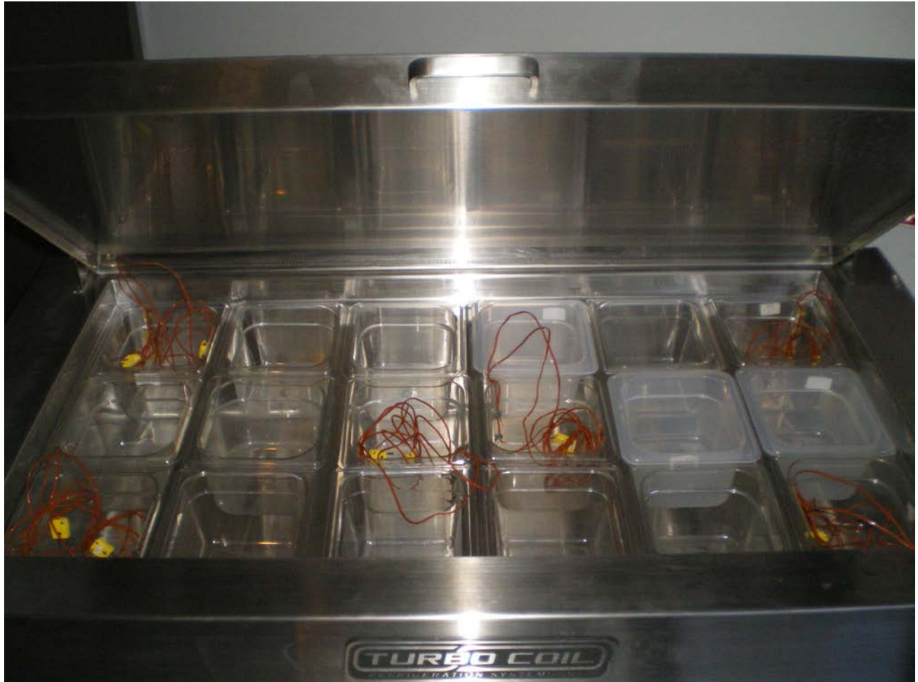
Turbocoil Pan Thermocouple Placement
