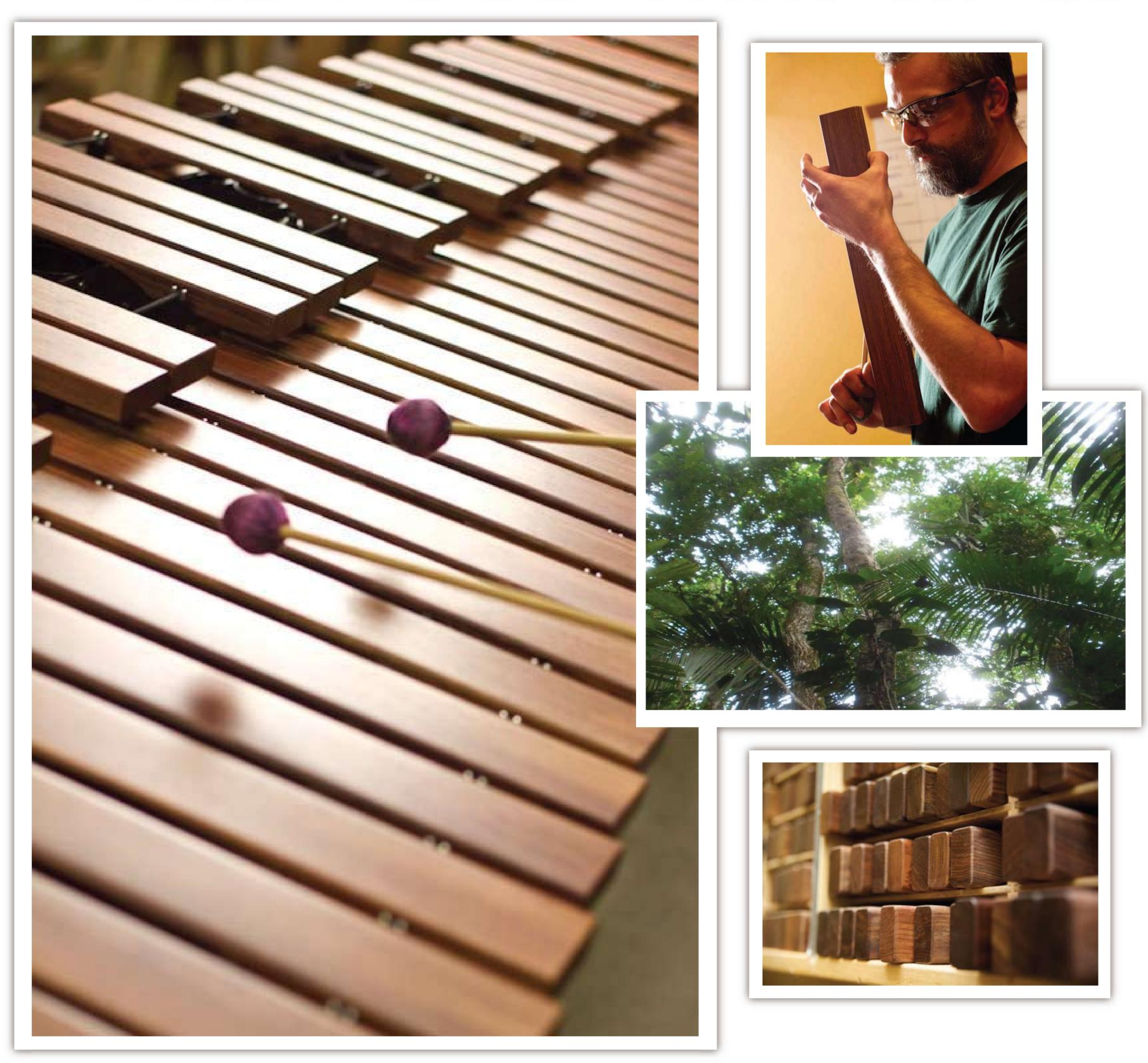
It starts with the wood selection: hand inspecting both faces and edges of every piece of rosewood for flaws. With over 100 sets of 5-octave bars to choose from, the master tuner can craft a keyboard with a cohesive sound that is dark, warm and resonant.
